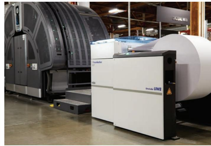
Top: The UW8 Unwinder feeds blank paper rolls into the HP T250 press at the front end of the inline Hunkeler Roll-to-Cut/Stack Solution. Below, finished booklets coming off Premier's Horizon SPF-200A Bookletmaker.
