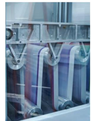
Hunkeler's WBB-L web buffer allows the press to keep running at full speed while the Hunkeler LS8-30 delivers stacks to the conveyor belt.
