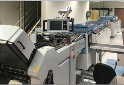
An in-line Hunkeler Roll-to-Stack system (R) provides the finishing for InfoSend's Canon inkjet press. A second near-line Hunkeler Roll-to-Stack/Roll-to-Fold solution with a Horizon folder (L) supports their Ricoh inkjet press. Both the Canon and Ricoh finishing lines include the Hunkeler DP8 II Dynamic Perforator, which performs dynamic perforation and punching in-line.
