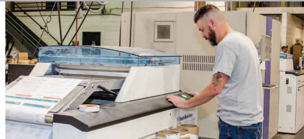
The high-speed Hunkeler unwinders and rewinders provide constant web tension for uniformly tight and straight rolls to ensure efficient, productive downstream processing on the Hunkeler Roll-to-Cut/Fold systems.
