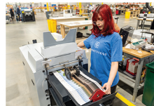
The Horizon C6F-362 Creaser/Folder, operated here by Nathaly Sarmiento, produces a wide variety of applications in the SC facility, saving valuable time and effort by creasing and folding in a single pass.
