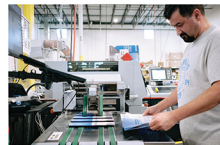
Operator Juan Diaz checks the quality of a finished booklet coming off the Horizon Stitch-Line Mark IV Saddlestitcher in MN. The system performs collating, scoring, folding, stitching, and trimming in one pass.
