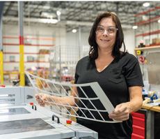
Running a 24-up business card application on the Horizon RD-N4055 Die Cutter in SC, operator Rhonda Clugston holds up the waste sheet that is automatically removed by the separator unit and delivered to the waste bin – no manual separation required.
