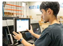
The touchscreen on the Horizon HF-300 Trimmer, which runs inline with the BQ-500 Perfect Binder in SC, helps make setup and changeover easy for operator Moises Birruet.
