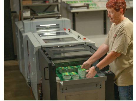
Stacked cards are unloaded from the Horizon RD-N4055 Rotary Die Cutting System, which has allowed Three Z to expand their business with new die-cut projects.
