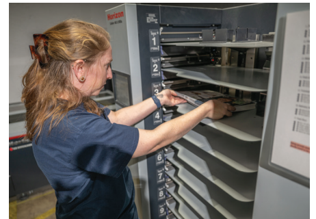
The Mark IV features two VAC-L1000 Collating Towers which provide flawless feeding on virtually any stock, at speeds up to 9,900 sets per hour. Above, sheets are loaded into one of the bins on the 10-station tower.
