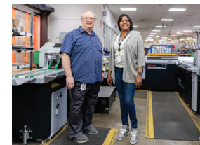
Wayne Pittillo (Operation Manager) and Charles Norman (Operation Director) work with the Horizon StitchLiner Mark III, an earlier generation saddlestitcher which outputs an average of 2,500 booklets/hour.
