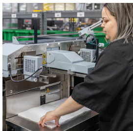
Sinthia Estrada loads the HSF-50 High-Speed Sheet Feeder connected to the new StitchLiner Mark V, which can feed up to 45,000 sheets/hour.
