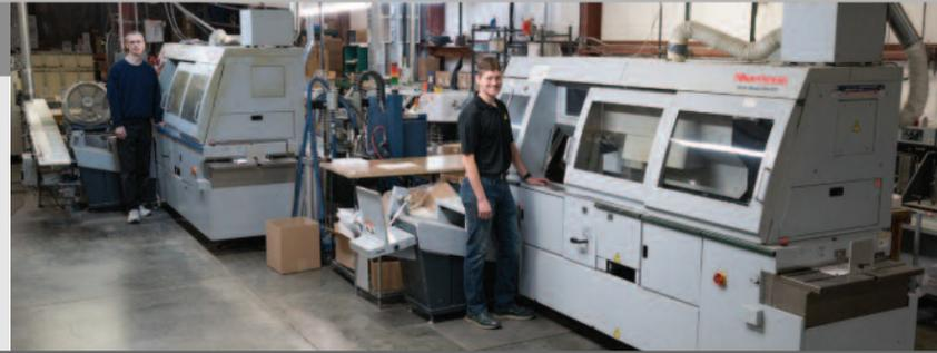
Two HT-70 Three-knife Trimmers (far right) round out the book manufacturing process with automated trimming of the perfect bound book blocks. For runs exceeding 700 books, Total Printing Systems employs the Standard Horizon CABS 4000 Perfect Binding System (near right), which can produce up to 4,000 finished books per hour in one process.
