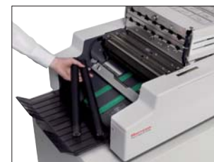
Lay the buckle section down and remove the rollers for cleaning or replacement.
