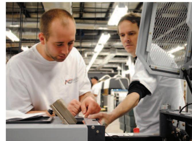
Tommy Greene, Digital Production Specialist and Mike Schaffer, Digital Finishing Specialist make final adjustments to the Standard Horizon Stitchliner 6000 Digital at AGS. Pre-printed rolls are converted to cut sheets and then booklets in a single pass with no touch points.
