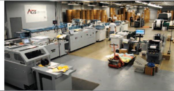
A Kodak Prosper 5000XL wide-web inkjet press has been complemented with a Standard Hunkeler PF7 Double Plow-Folder. A Standard Hunkeler UW6 Unwinder, a CS6 Cutter, and a Standard Horizon StitchLiner 6000 Digital makes for one lightning-fast saddlestitching workflow.
