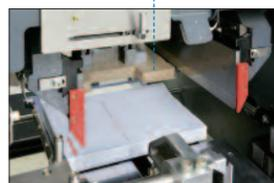
The height of each knife and the angle of the fore-edge knife can be adjusted through the color touch screen during operation. Trimmings are blown away from the knife by strong air nozzles mounted on the knife holders.
