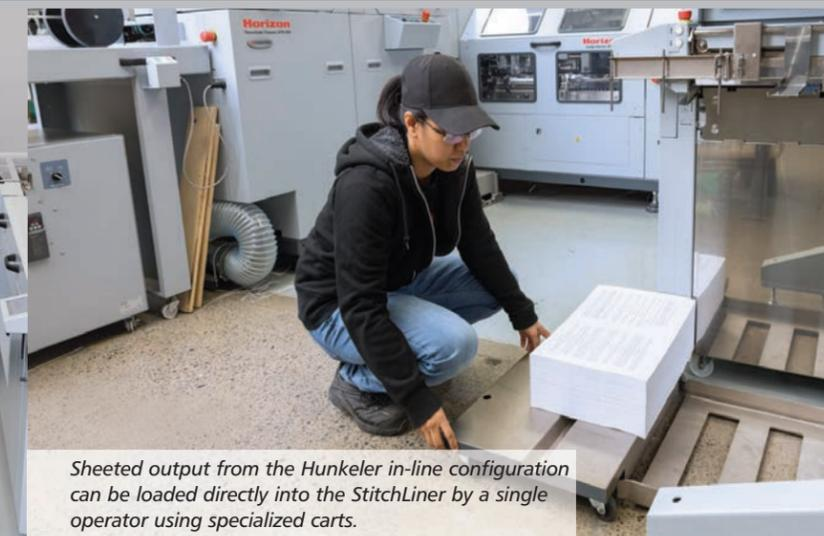
Sheeted output from the Hunkeler in-line configuration can be loaded directly into the StitchLiner by a single operator using specialized carts.
