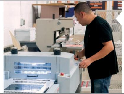
With the printed materials in place, Danny Ortiz, Digital Finishing Specialist, makes simple adjustments to the Standard Horizon RD-4055 Rotary Die Cutter before running the application.
