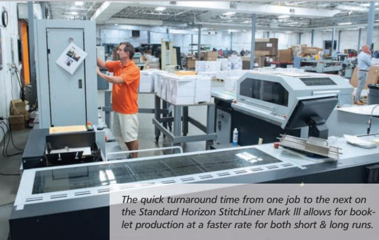
The quick turnaround time from one job to the next on the Standard Horizon StitchLiner Mark III allows for booklet production at a faster rate for both short & long runs.
