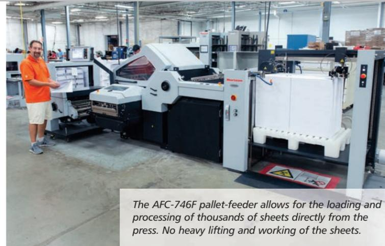
The AFC-746F pallet-feeder allows for the loading and processing of thousands of sheets directly from the press. No heavy lifting and working of the sheets.
