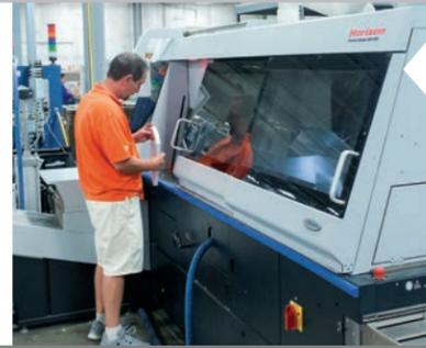
The BQ-480PUR has allowed Delzer to bring high-volume perfect binding capability in-house. The binder offers advanced automation including adjustments for roller height, nipping height, and amount of side glue.
