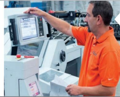
Changeovers and set-ups are quick and easy on the AFC-746F large-format folder using the intuitive, color, icon-based touchscreen. The system allows for up to 47 automated adjustments and runs 30% faster than its predecessor.
