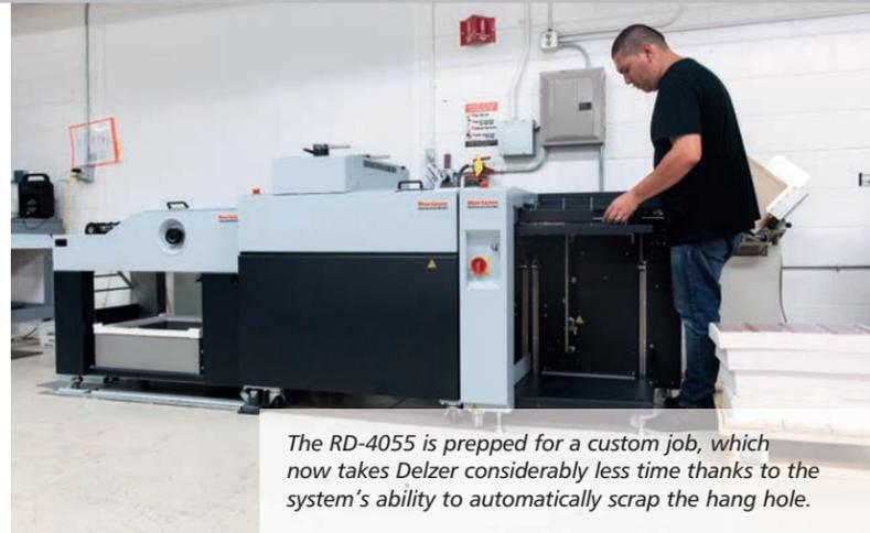
The RD-4055 is prepped for a custom job, which now takes Delzer considerably less time thanks to the system's ability to automatically scrap the hang hole.
