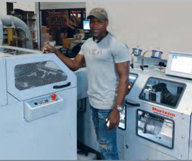
Lead Operator Paul Releford (left) operates the Standard Horizon StitchLiner 6000 Digital high-speed saddlestitcher integrated with Standard Hunkeler's UW6 Unwinder and CS6 Rotary Cutter, while Anna Benitez and Teresa Reyes (right) prepare finished booklets for shipping.
