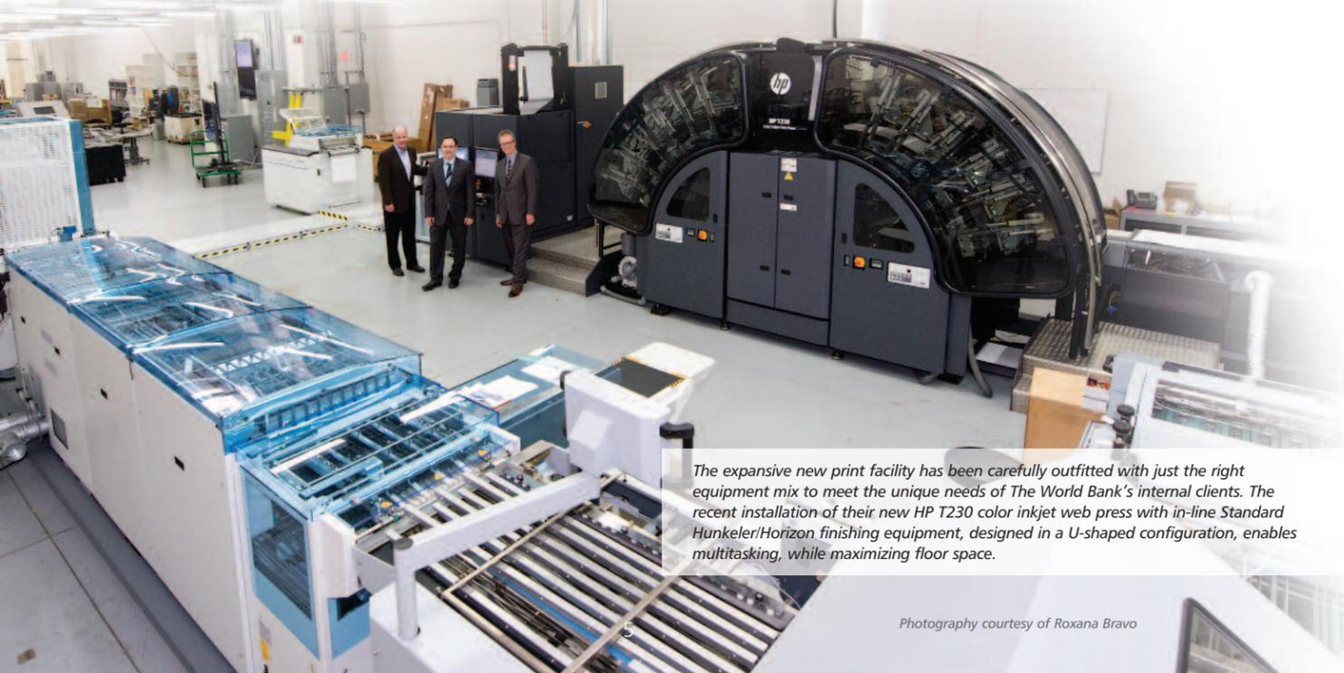
The expansive new print facility has been carefully outfitted with just the right equipment mix to meet the unique needs of The World Bank's internal clients. The recent installation of their new HP T230 color inkjet web press with in-line Standard Hunkeler/Horizon finishing equipment, designed in a U-shaped configuration, enables multitasking, while maximizing floor space.
