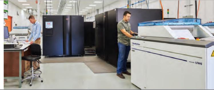
Depending on the nature of the job, printed rolls are transferred to one of two combination lines for book block production or processing into finished booklets on the Standard Horizon StitchLiner 6000 Digital Saddlestitcher (shown at right).
