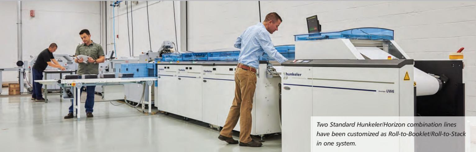
Two Standard Hunkeler/Horizon combination lines have been customized as Roll-to-Booklet/Roll-to-Stack in one system.
