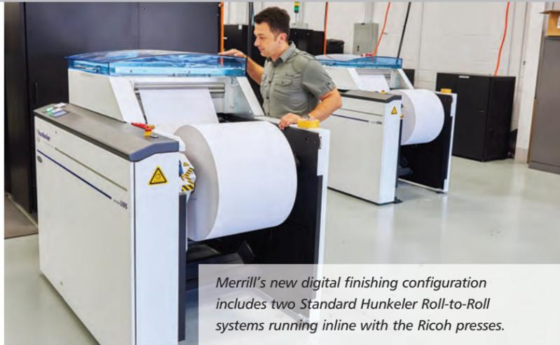
Merrill's new digital finishing configuration includes two Standard Hunkeler Roll-to-Roll systems running inline with the Ricoh presses.
