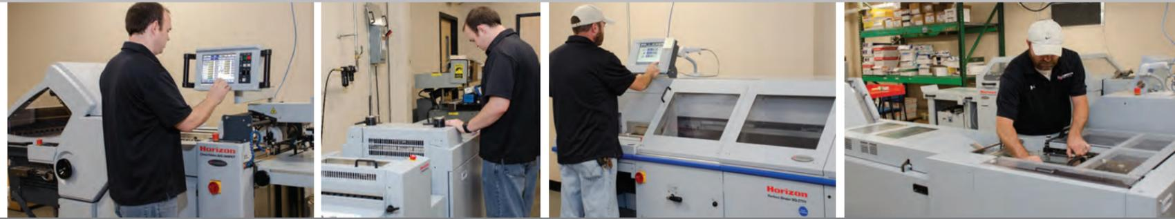
A Standard Horizon StitchLiner 5500 Saddlestitcher with HOF-400 Sheet Feeder processes digitally collated output from the HP presses into professionally finished booklets, while a BQ-270V Perfect Binder with HT-30 Three-side Trimmer is used to achieve high-quality on-demand production of variable thickness books.
