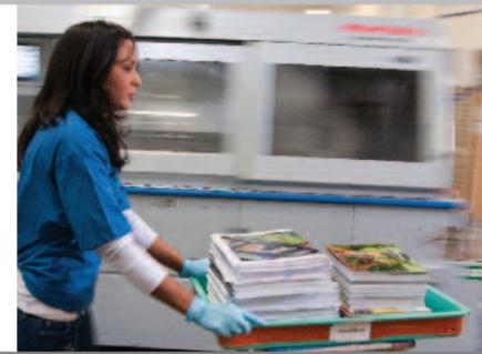
The Standard Hunkeler line consists of the UW6 unwinder, CS6-II cutter, SE6 separator, and an LS6 stacking module. Operators whisk perfect bound books from the Standard Horizon BQ-470 for final trimming.
