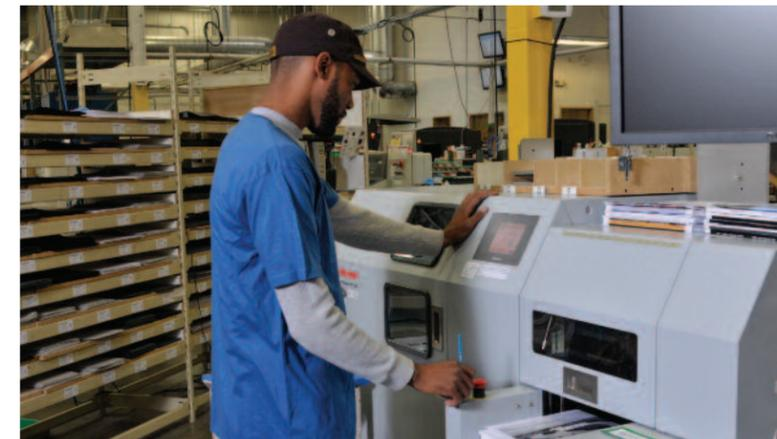
Once the book blocks are created on the Standard Hunkeler line and bound on the Standard Horizon BQ-470 perfect binder, they are loaded into the HT-30 for unattended three-side trimming.
