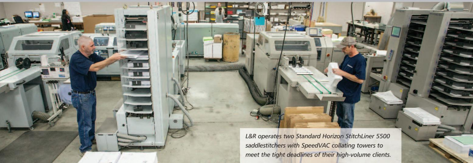
L&R operates two Standard Horizon StitchLiner 5500 saddlestitchers with SpeedVAC collating towers to meet the tight deadlines of their high-volume clients.
