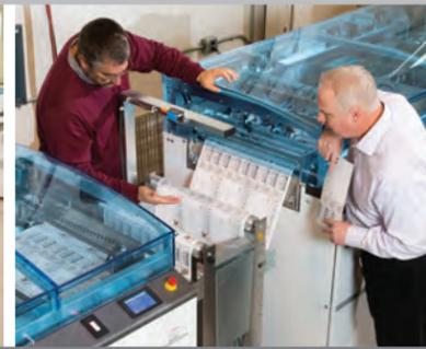
More recently, Heeter added an inline Standard Hunkeler Roll-to-Roll system, and a near-line Standard Hunkeler Roll-to-Stack system with a DP8-II Dynamic Perforating module (left). Printed rolls coming off the press are moved to the Roll-to-Stack system, and processed into book blocks with dynamic perforations throughout.
