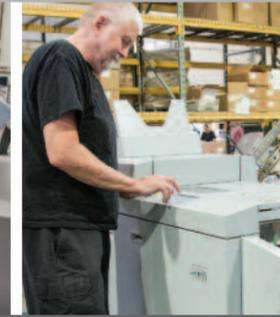
Maria Velasco operates the Standard Horizon StitchLiner 5500 Saddlestitcher with sheet feeding for digitally collated sets, while Ron Trydal works with one of two Standard Horizon CRF-362 Creaser/ Folders. These systems allow Darwill to take a stacked, collated set from any press through to finished booklets in a very efficient manner.
