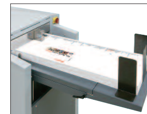
The support table for longer sheets is used when the sheet length is 650 mm / 25.5" or longer. The maximum sheet length which can be loaded is 865 mm / 34.0".
