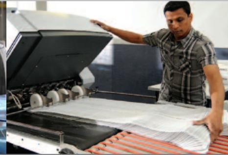
*The DIF-56 is significant, because it allows Access Direct to use the AF-566 Folder in-line with the complete finishing system to process roll-fed print, or off-line as a standalone device for processing cut-sheet work.*
