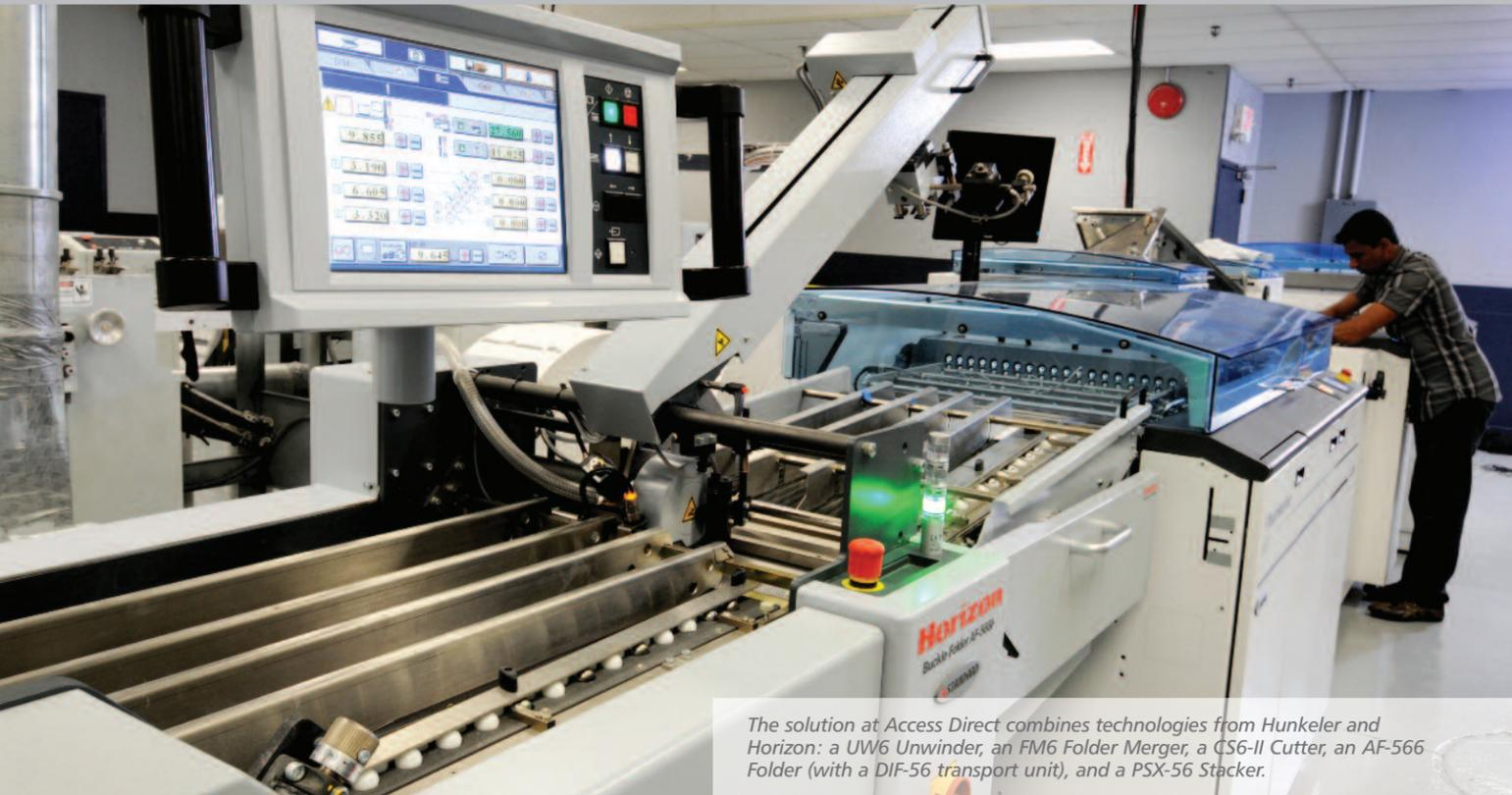
*The solution at Access Direct combines technologies from Hunkeler and Horizon: a UW6 Unwinder, an FM6 Folder Merger, a CS6-II Cutter, an AF-566 Folder (with a DIF-56 transport unit), and a PSX-56 Stacker.*
