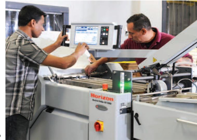
*The advanced folder automation and touchscreen control allows ultra-quick set-ups in the Access Direct production facility.*
