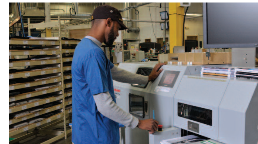
Once the book blocks are created on the Standard Hunkeler line and bound on the Standard Horizon BQ-470 perfect binder, they are loaded into the HT-30 for unattended three-side trimming.
