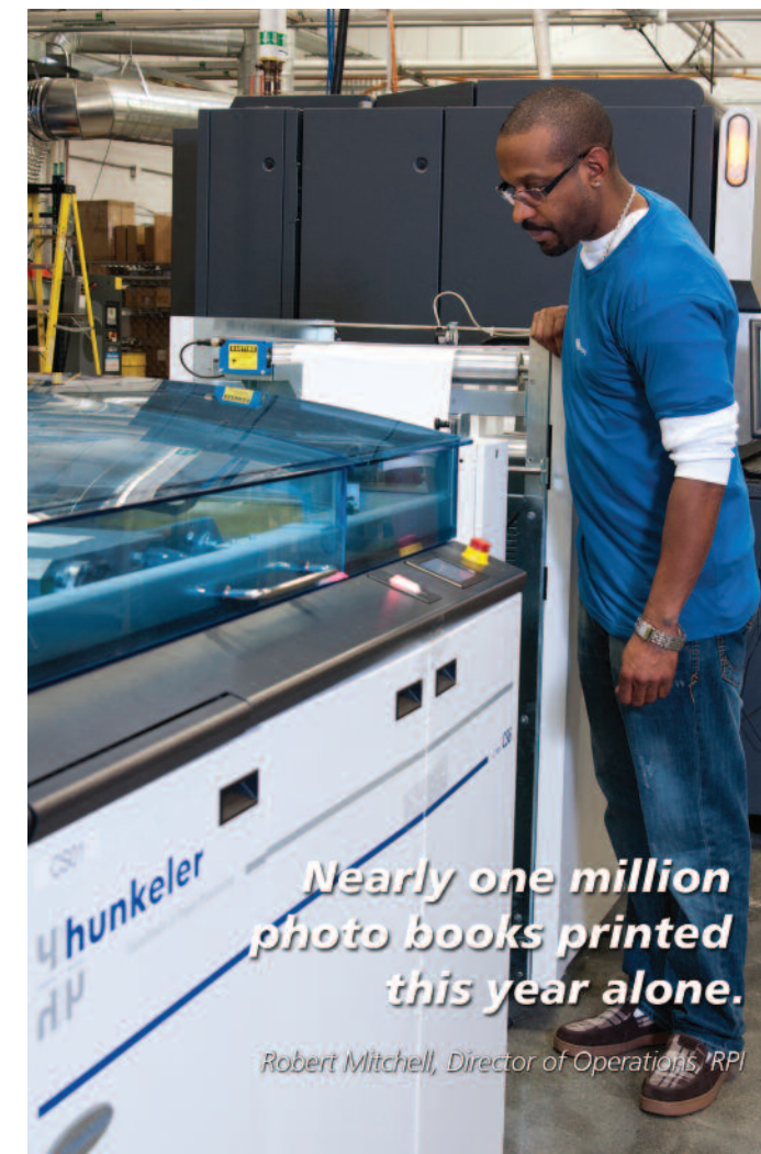
Once the book blocks are created on the Standard Hunkeler line and bound on the Standard Horizon BQ-470 perfect binder, they are loaded into the HT-30 for unattended three-side trimming.
